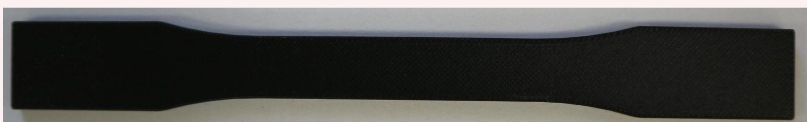
Fig. 1 Tensile test sample made of PLA
