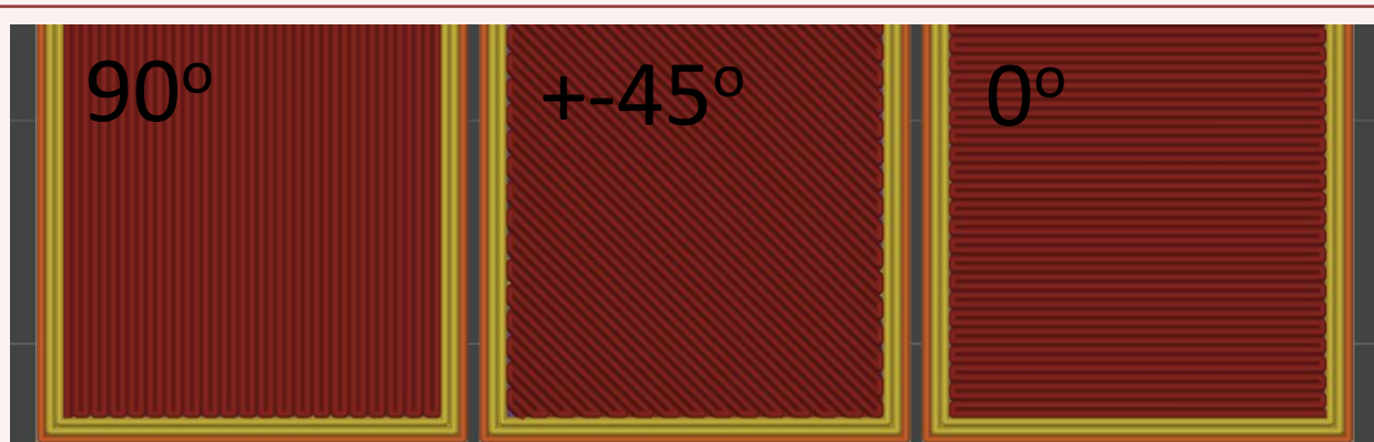
Fig. 1 Layer Orientation in the slicer
